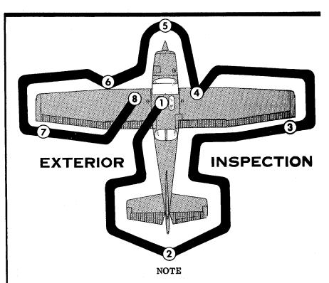
Visually check aircraft for general condition during walkaround inspection. In cold weather, remove even small accumulations of frost, ice or snow from wing, tail and control surfaces. Also, make sure that control surfaces contain no internal accumulations of ice or debris. If night flight is planned, check operation of all lights, and make sure a flashlight is available.
